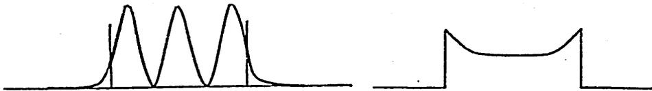
(b) Multi-peaked intensity distribution Three peaks are assumed to be in-phase in the field. (d) Obtained steady-state refractive index distribution
