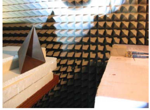
Fig. 2. Photograph of the trihedral corner reflector that was measured using the two Vivaldi antennas.
