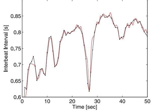
Fig. 15. IBIs estimated from the ECG (black) and the radar signal (red) using the proposed method for participant 2.
