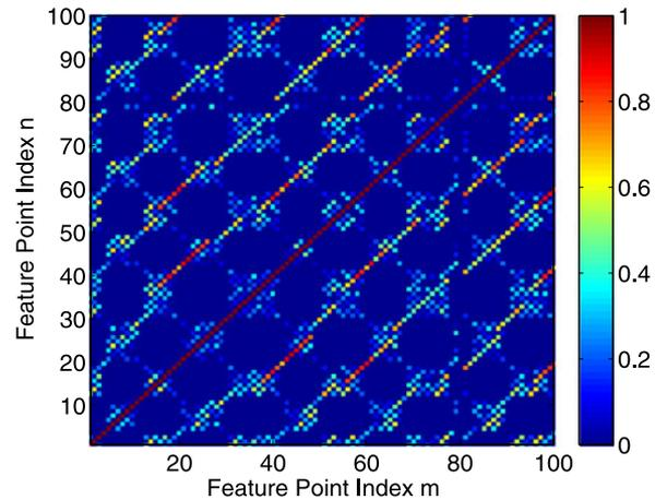
Fig. 12. Self-similarity matrix of feature topology signal using the proposed phase assignment, as shown in Fig. 9.
