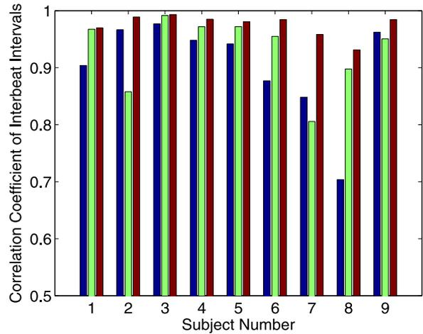
Fig. 24. Correlation coefficients of IBIs estimated from the radar signal and ECG data. The proposed method (in red) with  $(\theta_c, \theta_t) = (0.1, 0.7)$ , is compared with the correlation-based methods with  $(\theta_c, \theta_t) = (0.1, 0.0)$  (in blue) and  $(\theta_c, \theta_t) = (0.7, 0.0)$  (in green).
