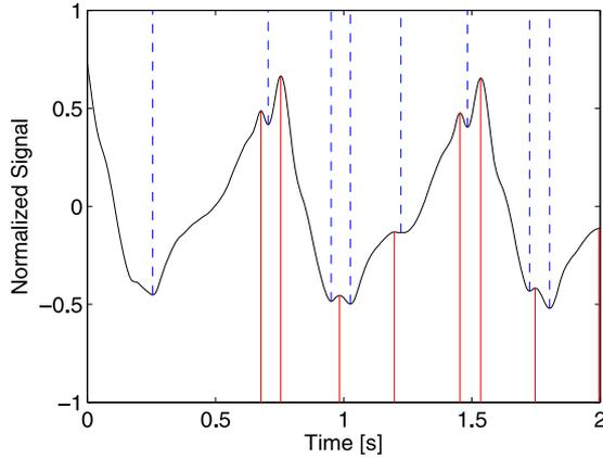
Fig. 4. Radar signal  $s(t)$  with feature points of PKs (solid red lines) and VLs (dashed blue lines).
