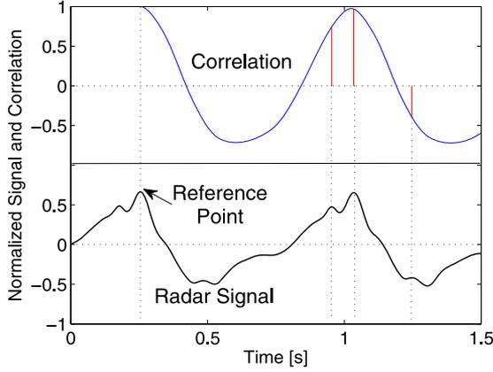
Fig. 6. Radar signal (lower black curve), its local autocorrelation function (upper blue curve) and correlation coefficients evaluated using the proposed method (red lines).
