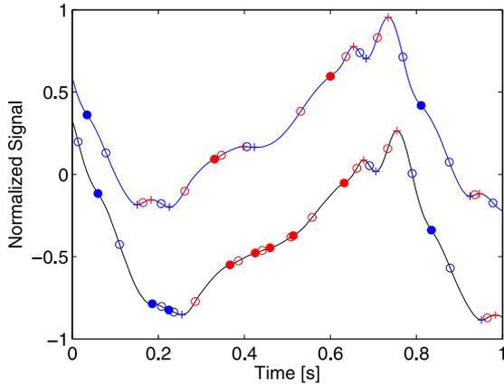
Fig. 7. Radar signal and feature points. PK, VL, RDP, RDPV, FDP, and FDV are marked with a red cross, a blue cross, a red circle, a red-filled circle, a blue-filled circle, and a blue circle, respectively.
