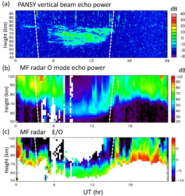
Fig. 3. A typical example of winter echoes, observed on 22 April 2015. (a) The echo power of the vertical beam by the PANSY radar, (b) O mode echo power by the MF radar, and (c) the ratio of E mode echo power to O mode echo power by the MF radar. Sunrise and sunset times at each altitude are indicated by the dashed lines.
