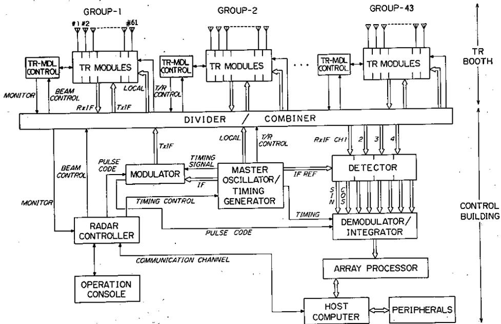
Fig. 2. General block diagram of the equatorial radar.
