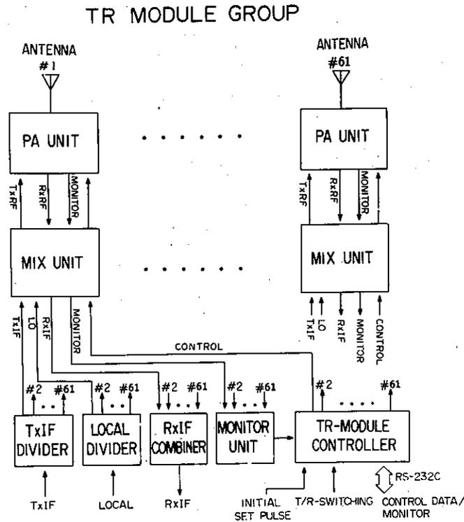
Fig. 3. Block diagram of one group of TR modules.
