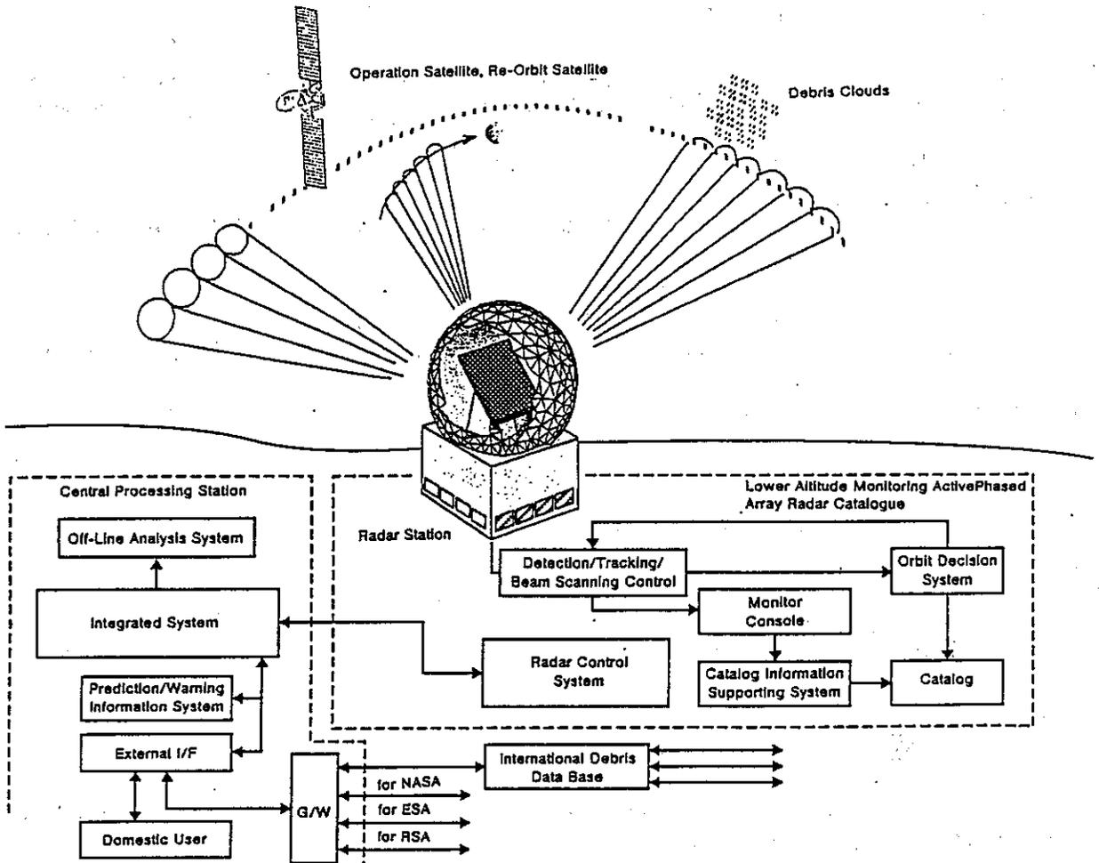
Fig.7. Concept of the space debris radar of NASDA.
