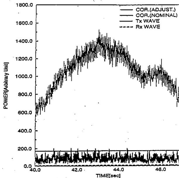
Fig.3. Time change of the carrier level.
