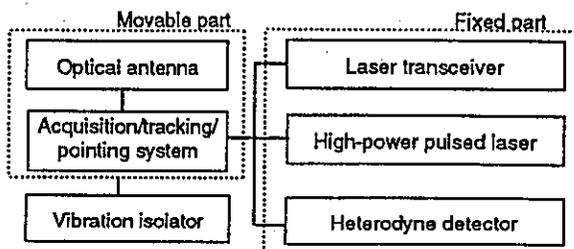
Fig.5. Optical/mechanical part of the onboard transponder.
