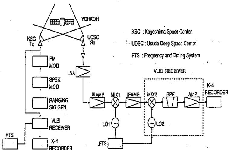
Fig.1. Configuration of the bistatic radar.
