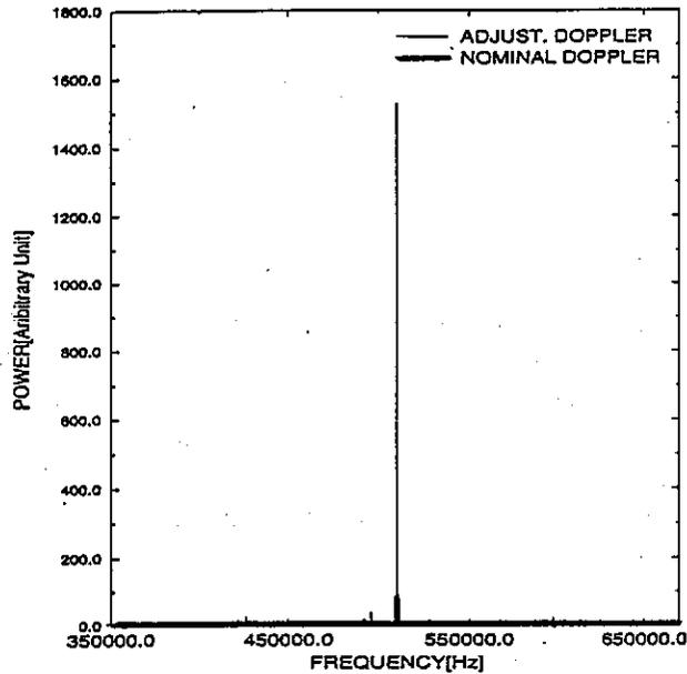
Fig.2. Correlated spectrum with/without Doppler compensation.
