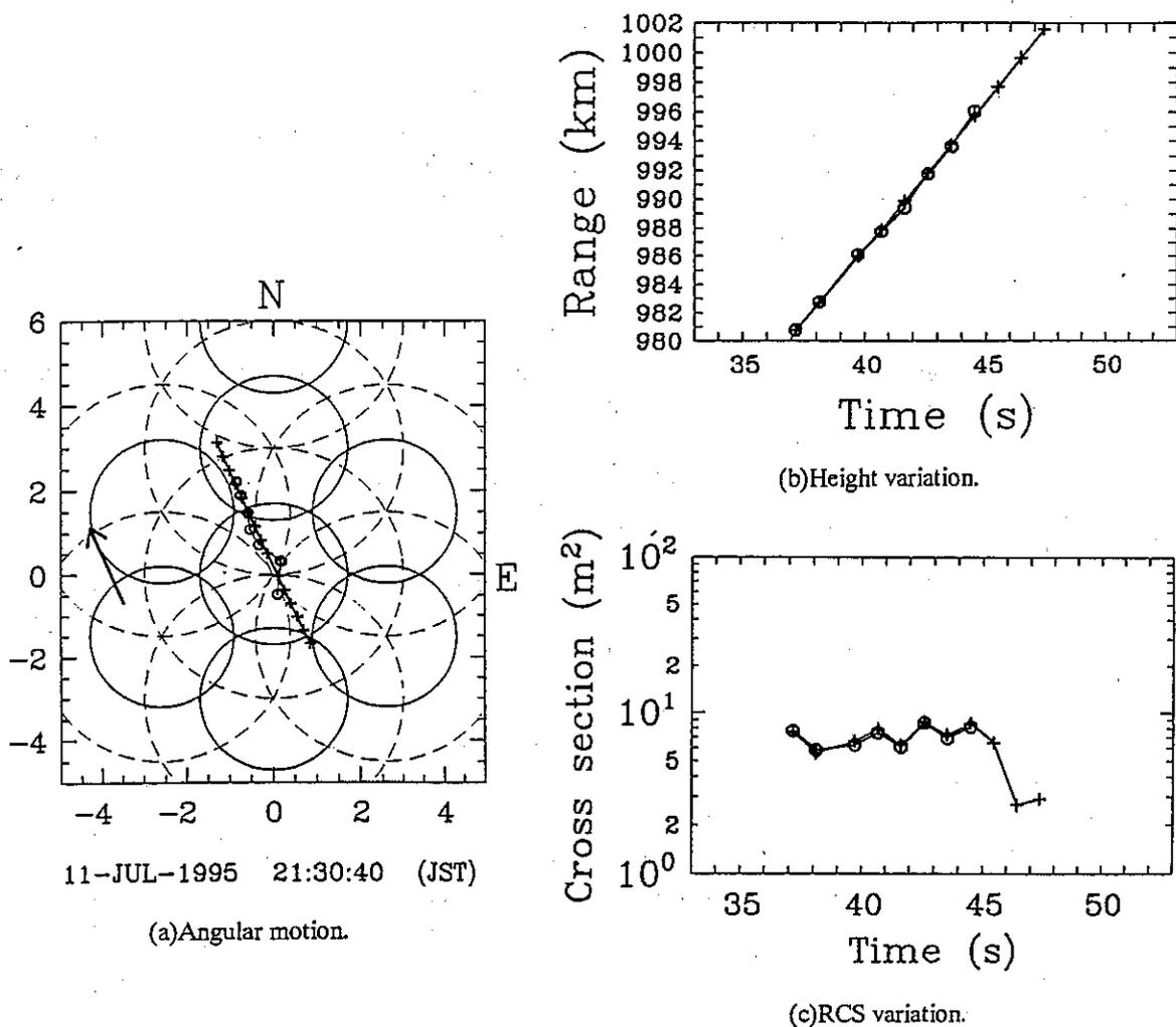
Fig. 4. MU radar observation data of MOS-1b.
