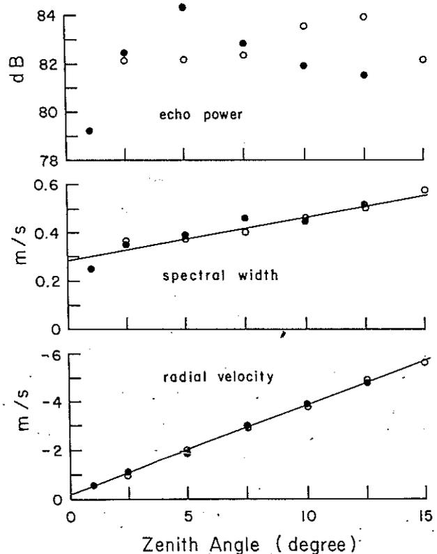
FIG. 4. The echo power, spectral width and radial velocity versus zenith angle. The zenith angle was changed from  $15^\circ$  to zero (open circles), then back to  $12.5^\circ$  (solid circles). All the measurements were done within about 70 min.
