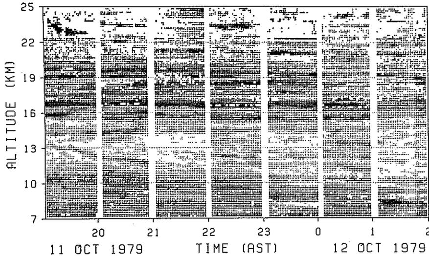
FIG. 2. 8-level height-time shade plot of the echo power. The dynamic range is 32 dB. Missing points due to poor quality of data left blank.
