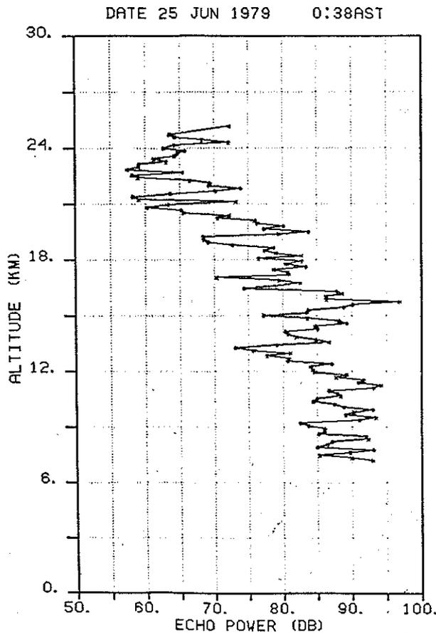
FIG. 1. The received echo power versus height (after Sato and Woodman, 1980). The noise level is about 59 dB.
