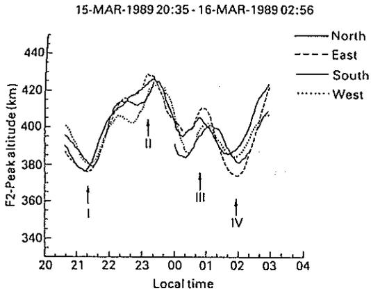
Fig. 3. Temporal variations of the  $F_2$  peak altitude obtained by MU radar multiple beam observations performed during the night of 15–16 March 1989. The thick solid line is for the north oblique beam, the thick dotted line for the east beam, the thin solid line for the south beam and the thin dotted line for the west beam. I, II, III and IV show ionospheric disturbances.
