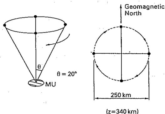
Fig. 1. Schematic diagrams of the beam directions used in the MU radar multiple beam observations. The antenna beam is sequentially steered to four oblique directions (magnetic north, east, west and south), at a zenith angle of 20°. With this configuration the distance between scattering volumes in each beam position is 200-300 km at the *F*-region altitudes.
