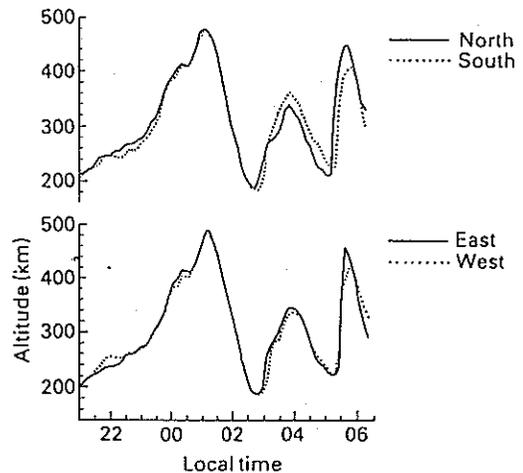
Fig. 5. Temporal variations of the height  $z_L$  at which the electron density is  $6 \times 10^4 \text{ cm}^{-3}$ , obtained by the multiple beam observation during the night of 20–21 January 1989. The height  $z_L$  corresponds to the minimum virtual height ( $h'F$ ) of the  $F$ -layer. The top plot shows the data in the north (solid line) and south oblique (dotted line) beams. The bottom plot shows the data in the east (solid line) and west oblique (dotted line) beams.
