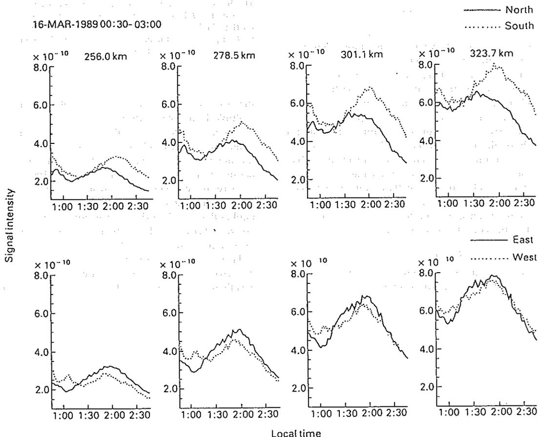
Fig. 2. Temporal variations of signal powers obtained by the MU radar multiple beam observation performed after midnight on 16 March 1989. The top four plots show the data in the north (solid line) and south oblique (dotted line) beams at heights of 256, 278, 301 and 323 km. The bottom four plots show the data in the east (solid line) and west oblique (dotted line) beams at the same height as the plots above.
