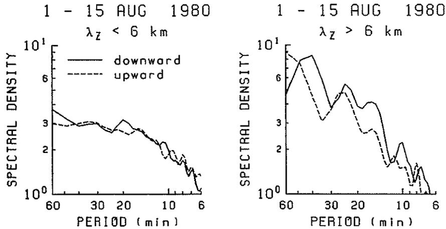
Fig. 8. Frequency power spectra of the wind fluctuations on the vertical scale larger (right) and smaller (left) than 6 km. The abscissa represents periods. Solid and dashed lines indicate the downward and upward phase propagations, respectively.
