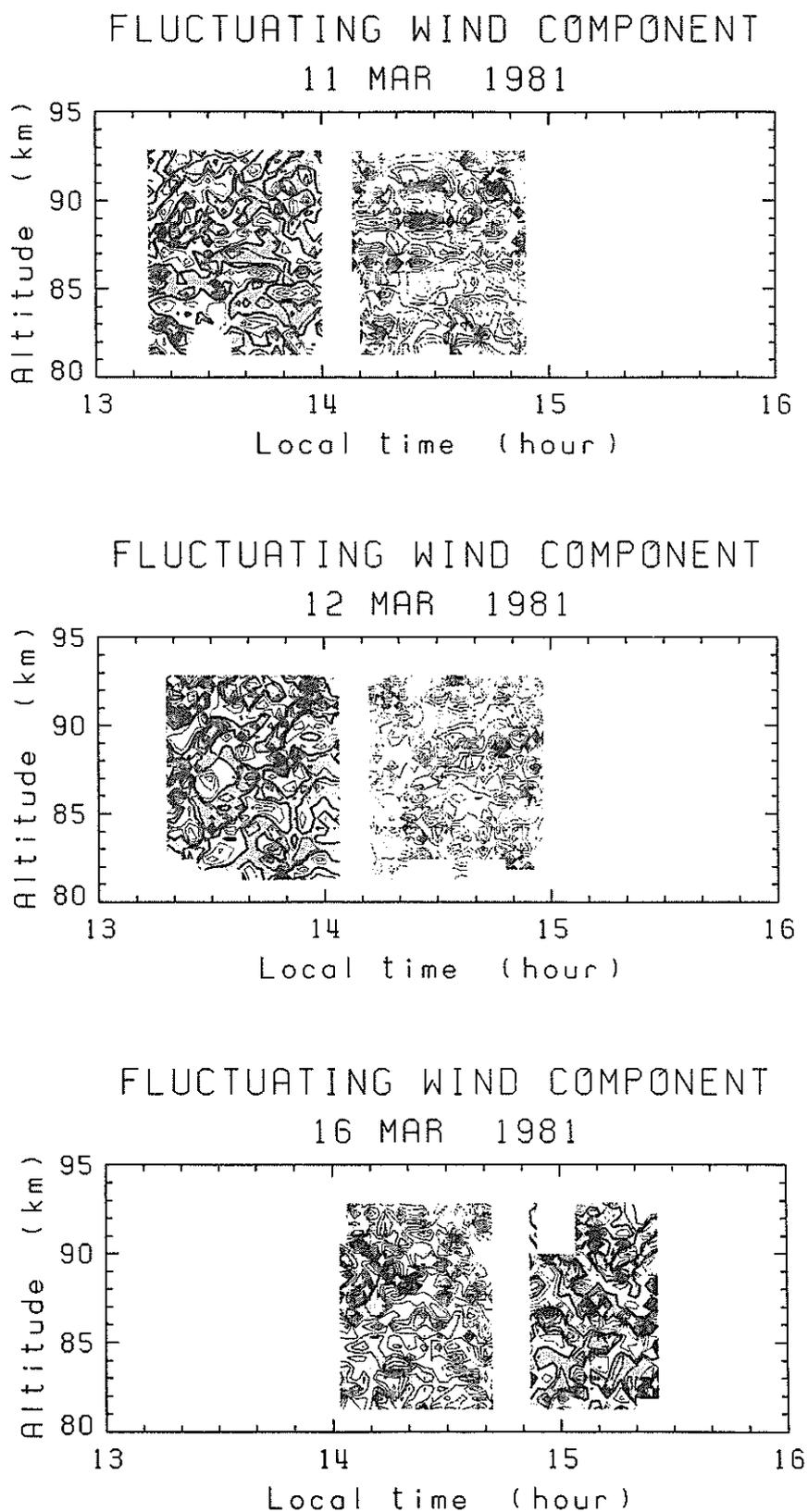
Fig. 6. Wind fluctuations with vertical scale smaller than 6 km observed on March 11, 12, and 16, 1981. No time filter is applied. Zonal component is shown by dark-shaded area, and meridional by light-shaded area.
