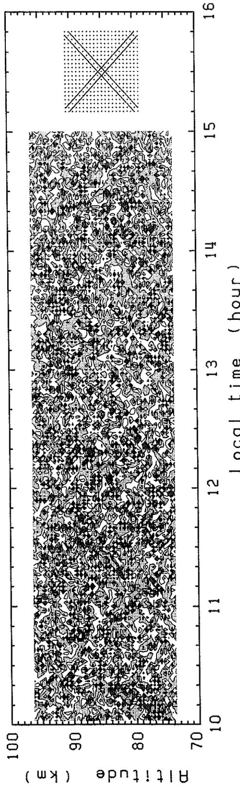
Fig. 4. A time-height section of computer-generated random fluctuation with standard deviation of  $2 \text{ m s}^{-1}$  analyzed in the same way as in Figure 3. The contour intervals are  $2 \text{ m s}^{-1}$ . Dot pattern near the right edge of the diagram indicates some of the data points, while thin solid lines are the diagonal lines of the data points (see text).
