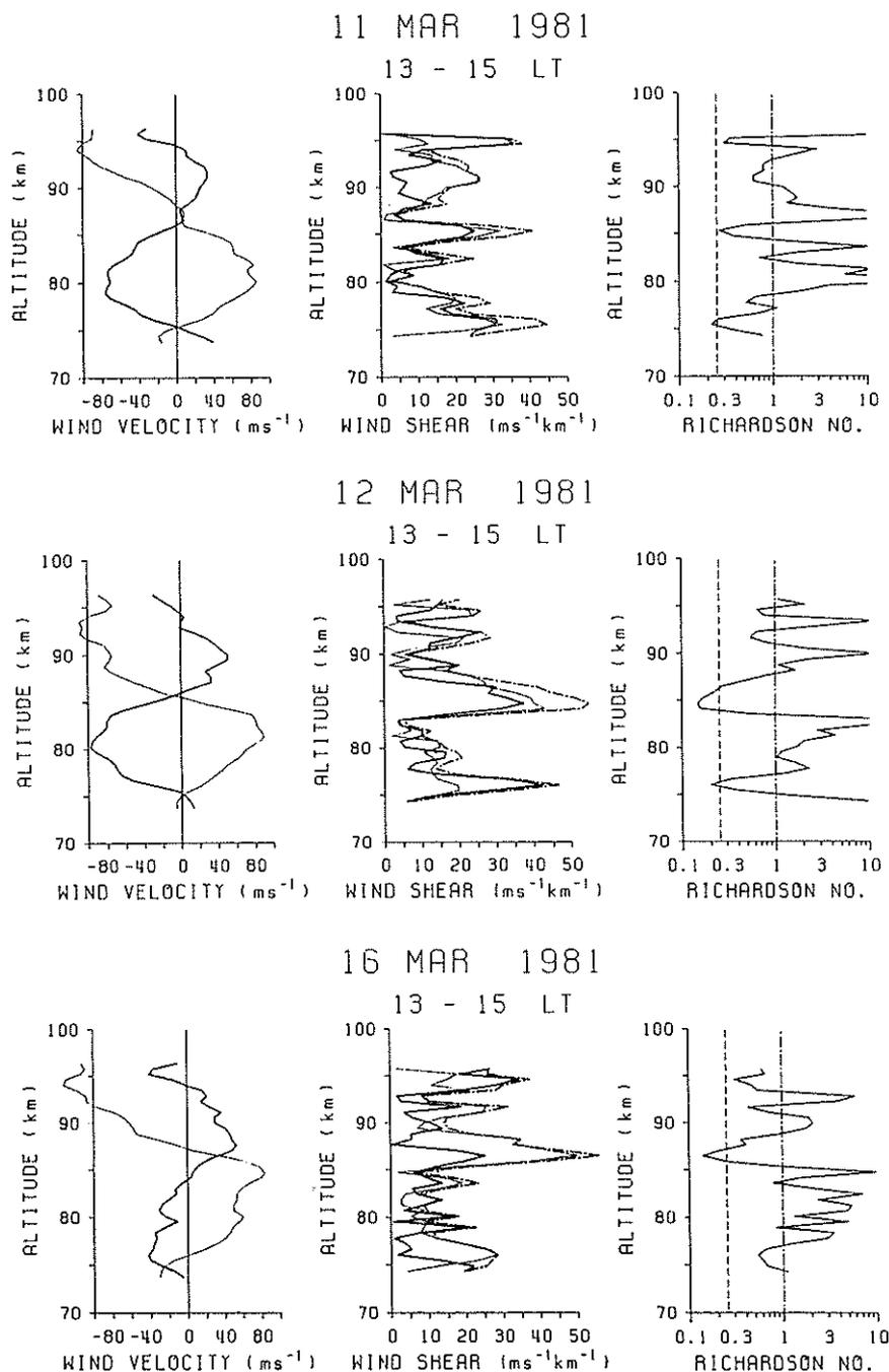
Fig. 9. Hourly profile (left) and vertical shear (center) of the horizontal wind, observed on March 11, 12, and 16, 1981. A deduced Richardson number is shown on the right for the Brunt-Väisälä period of 5 min. Thick and thin lines are zonal and meridional components, respectively, while dot-dashed lines show the absolute shear of the horizontal wind.
