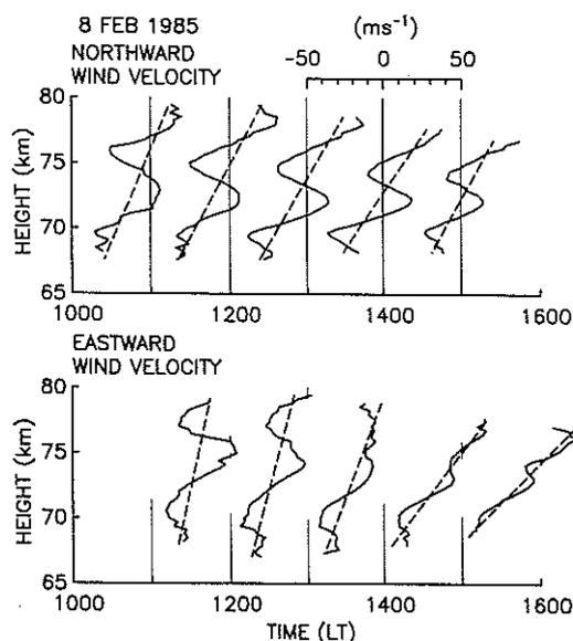
Fig. 1. Northward (top) and eastward (bottom) wind profiles observed on February 8, 1985. Each profile is averaged over 2 hours with 1 hour overlap. Dashed lines show linear trends of each wind profile.
