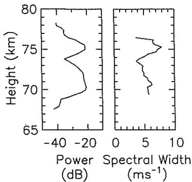
Fig. 9. Profiles of echo power (left panel) and spectral width (right panel) averaged over 1230-1330 LT on February 8, 1985.
