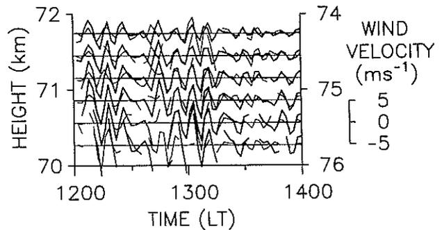
Fig. 5. Radial wind variations at altitudes the same distances above and below the phase reversal height (73 km), with the sign of one reversed. Thick lines show the variations below 73 km with receding positive, and thin lines show those above 73 km with approaching positive. The left and right vertical axes show the altitudes below and above 73 km, respectively.
