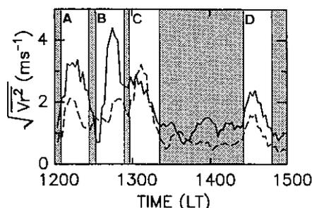
Fig. 6. Variation of rms speed of the radial wind fluctuations  $\sqrt{V_r^2}$  in Figure 4 averaged in the altitude range of 70–72 km (solid line) and 74–76 km (dashed line). A, B, C, and D show events of large fluctuations which occur during 1205–1227, 1232–1254, 1258–1321, and 1424–1446 LT, respectively.
