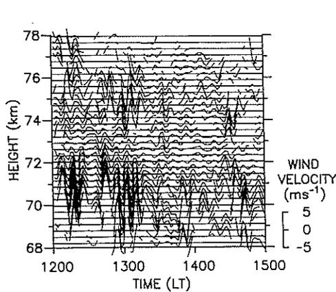
Fig. 4. Radial wind fluctuations with periods ranging from 6 to 16 min observed in the southward beam on February 8, 1985.
