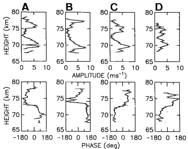
Fig. 7. Amplitude (top) and phase (bottom) profiles of the radial wind fluctuations obtained in each event shown in Figure 6. Radial wind velocities are fitted by assuming a sinusoidal oscillation with a period of 9 min. Error bars on the profile indicate the standard deviation of the estimated amplitudes and phases.
