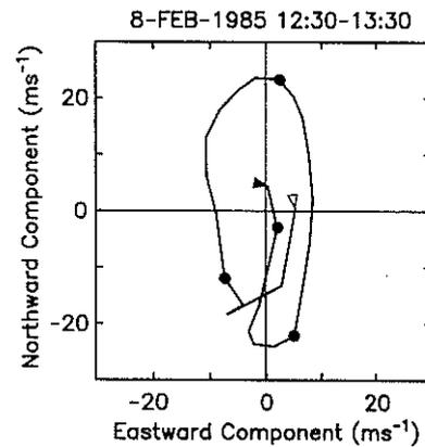
Fig. 2. A polar plot of the wind velocity averaged over 1230–1330 LT on February 8, 1985. Vertical linear trend of the wind profile is subtracted. The open and solid triangles on the solid line indicate the lowest (68.8 km) and highest altitudes (76.5 km). Circular symbols are plotted at 70, 72, 74, and 76 km.
