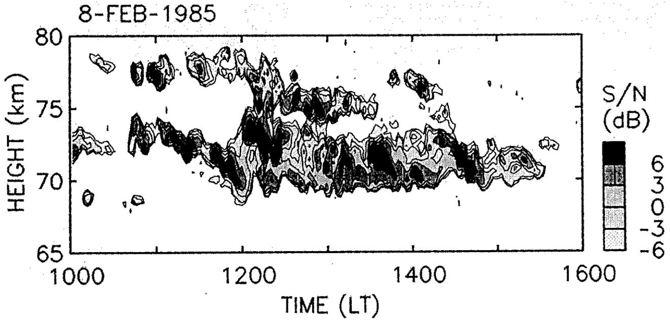
Fig. 8. Time-height sections of the signal to noise ratio observed in the southward beam on February 8, 1985.
