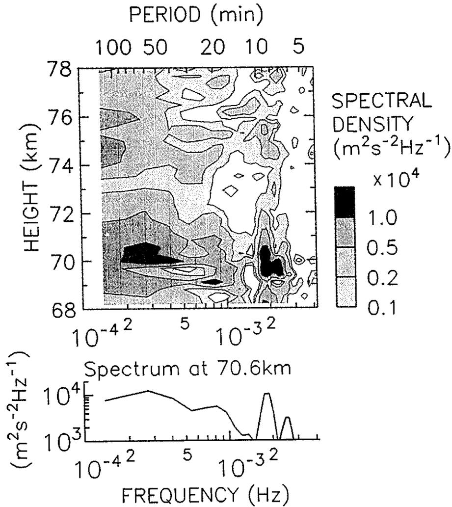
Fig. 3. The top panel shows the height distribution of power spectral densities of radial wind fluctuations observed during 1000–1600 LT in the southward beam on February 8, 1985. The bottom panel shows the power spectrum obtained at 70.6 km.
