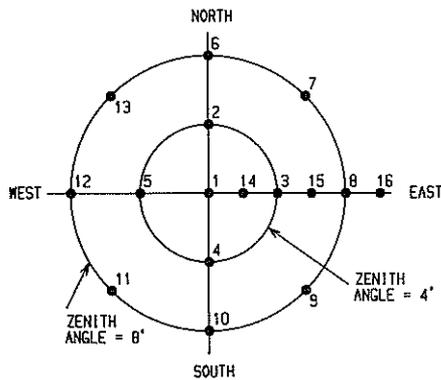
Fig. 1. Schematic top view of the antenna directions.
