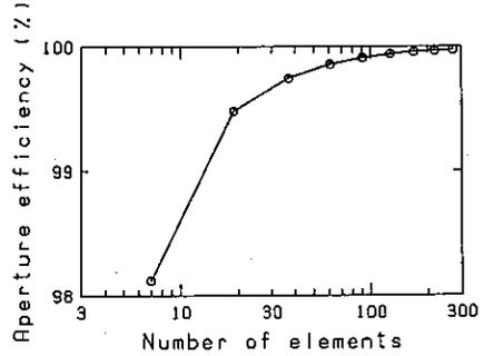
Fig. 11. The aperture efficiency of the array versus array size. The small circles show the calculated values for hexagonal arrays with elements of 7, 19, 37, 61, 91, 127, 169, 217, and 271, respectively.
