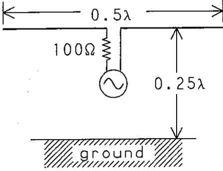
Fig. 3. Geometry of the half-wave dipoles.
