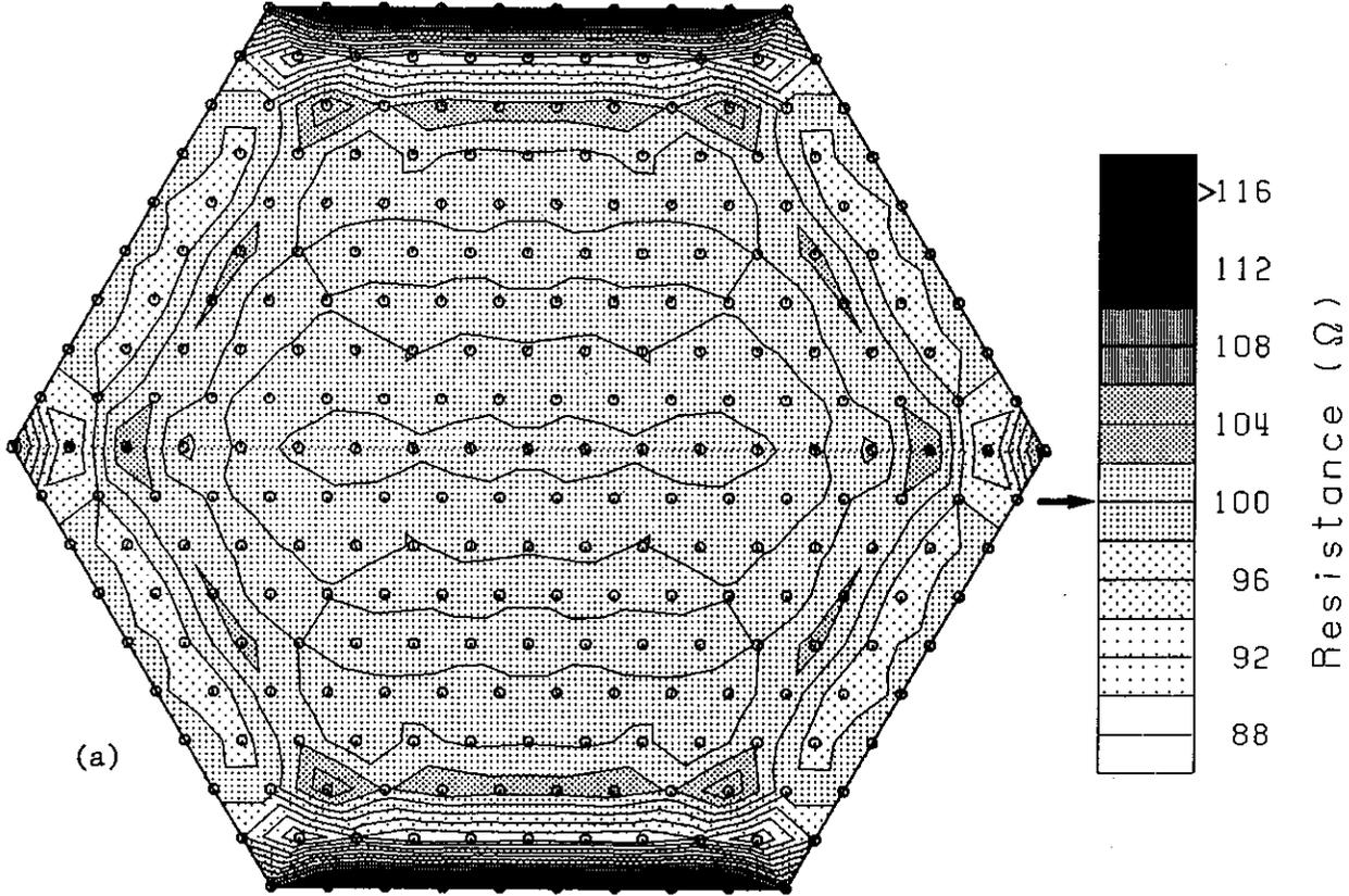
Fig. 5. Spatial variation of (a) active resistance, (b) active reactance and (c) array element gain shown in the form of a contour map. The element positions are shown by small circles, and the dipole direction is parallel to the bottom edge of the array. The arrow put on the contour scale on the right-hand side of each map indicates the values for the infinite array element.
