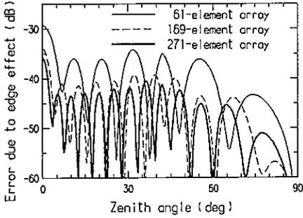
Fig. 9. Difference of the field intensity in the  $H$  plane between the exact solution and that obtained with infinite array approximation for three hexagonal arrays with different size. The difference is normalized to the main lobe field intensity of the respective arrays.
