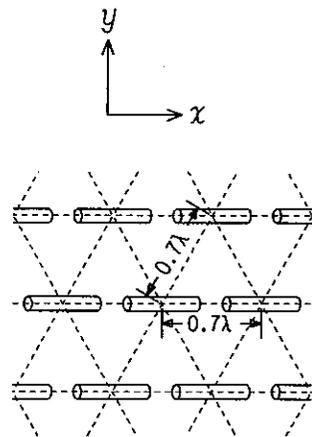
Fig. 2. The finite hexagonal array composed of 271 elements which are arranged on equilateral triangular grids with element spacing of  $0.7\lambda$  ( $\lambda$  is wavelength). Consecutive numbers are put in the element positions. Encircled elements will be discussed later.
