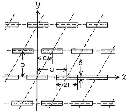
Fig. 1. Geometry of the infinite planar array with dipoles arranged on a general triangular grid. The dipoles are represented by equivalent thin sheets of width  $\delta$  and length  $2r(2r = \lambda/2; \lambda$  is wavelength).
