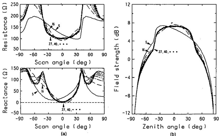
Fig. 6. (a) Active impedance and (b) array element pattern ( $H$  plane) for the ten elements encircled in Figure 2. They are shown by solid (5th) and dashed (16th) lines, one-point chain (27th), two-point chain (40th), etc. for the element order approaching the center from the edge of the array.
