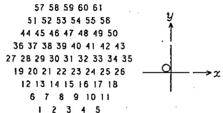
Fig. 2. (left) Hexagonal array composed of 61 Yagi antennas which are arranged on equilateral triangular grids with element spacing of  $0.7\lambda$  ( $\lambda$  is wavelength). Consecutive numbers represent the element positions. (right) Top view of a Yagi antenna and the coordinate system.
