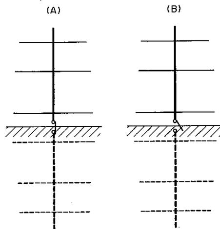
Fig. 6. Antenna mast and ground plane. (A) Antenna mast is earthed on a perfectly conducting ground, and (B) the ground plane is a perfect conductor, but the antenna mast is not earthed on it.
