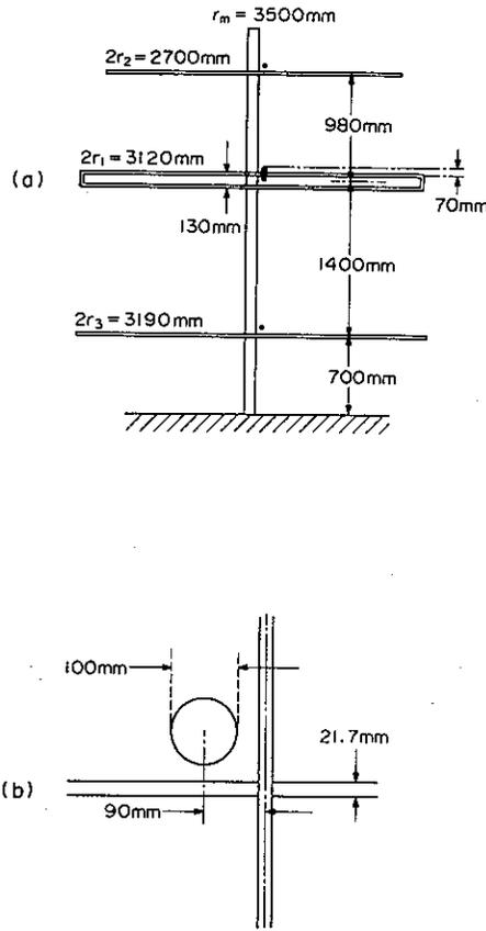
Fig. 1. (a) Front view of the crossed 3-subelement Yagi antenna used for the MU radar antenna;  $2r_i (i = 1, 2, 3)$  is subelement length and  $r_m$  is height of the antenna mast. Height difference between a pair of crossed subelements is 70 mm. (b) Top view of the same antenna illustrated only in the vicinity of the mast.
