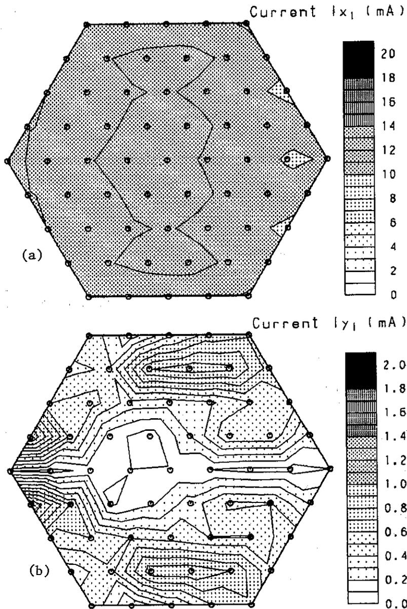
Fig. 7. Spatial current variations for case (A) in Figure 6. Current amplitudes on excited subelements ( $I_{x_1}$ ), subelements orthogonal to the excited ones ( $I_{y_1}$ ) and antenna masts ( $I_p$ ) are depicted in 7a, 7b and 7c, respectively.
