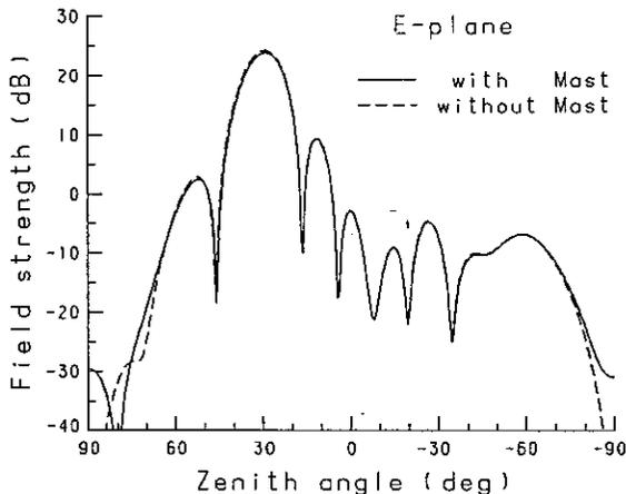
Fig. 8. Similar to Figure 5 except for comparison of array pattern between the cases with antenna masts (solid line) and without them (dashed line) for case (A) in Figure 6.
