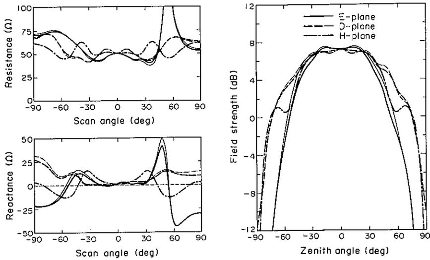
Fig. 9. Similar to Figure 4 except that comparison is made for the 29th element between the cases with (thick lines) and without (thin lines) antenna mast for case (A) in Figure 6.
