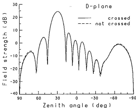
Fig. 5. Comparison of array pattern between the cases with the orthogonal subelements (solid line) and without them (dashed line). The abscissa is the zenith angle, while the ordinate is the electric field intensity over the radiation field of an isotropic antenna. The antenna beam is scanned by  $30^\circ$  off from the zenith in the  $D$  plane.
