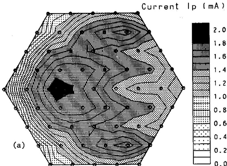
Fig. 10. (a) Spatial variation of mast current and (b) array pattern for case (B) in Figure 6. Array patterns with and without mast effects are represented by solid and dashed lines, respectively.
