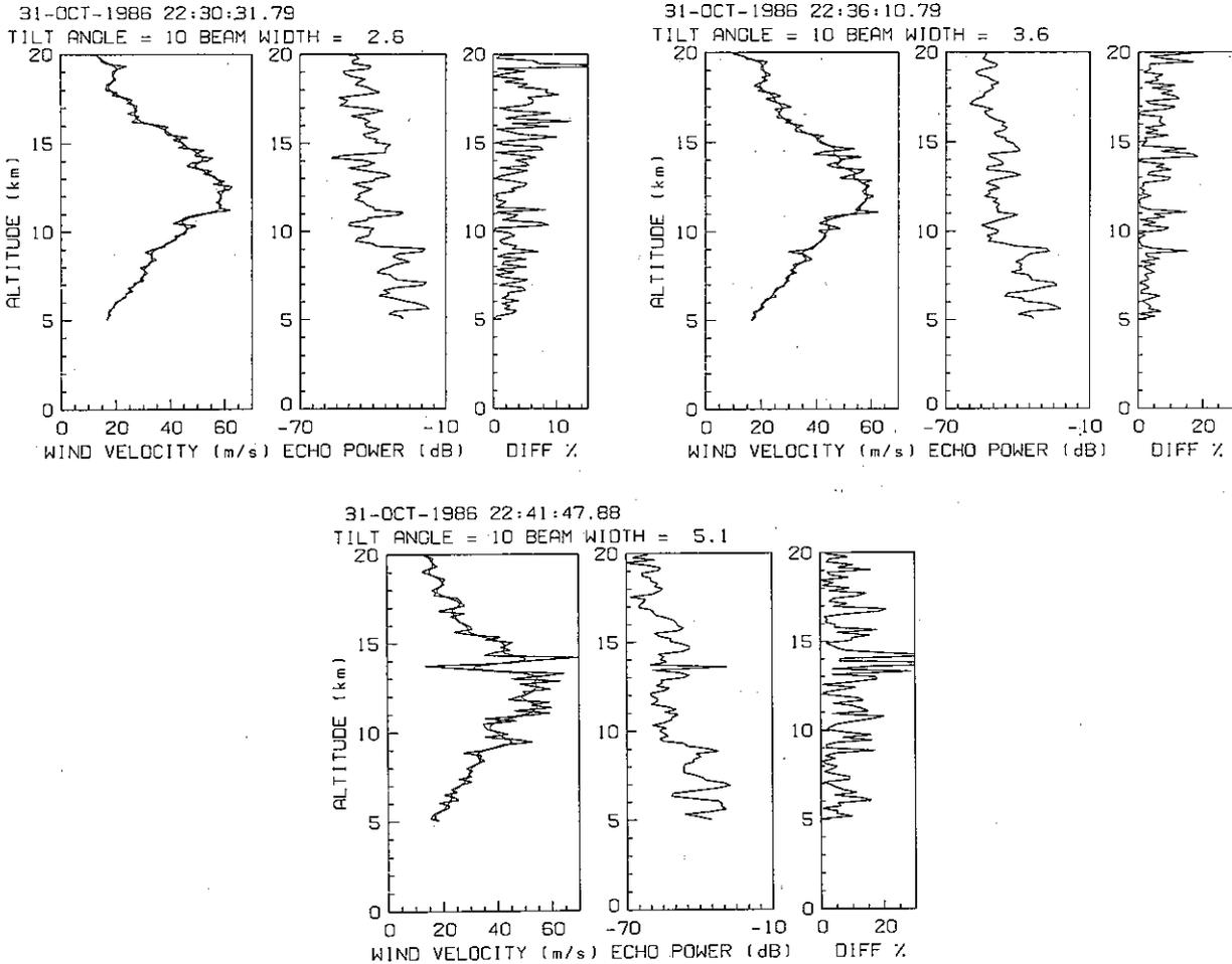
Fig. 4. MU radar observations, showing a single measured wind profile (zonal component) versus height together with a profile smoothed by two passes of a three-point running mean for various antenna beam widths (see text). The profile of echo power and the percentage difference between the measured and smoothed curves is also shown. The beam width is the two-way 3-dB beam width, and the height resolution is the range weighting function 3-dB width.
