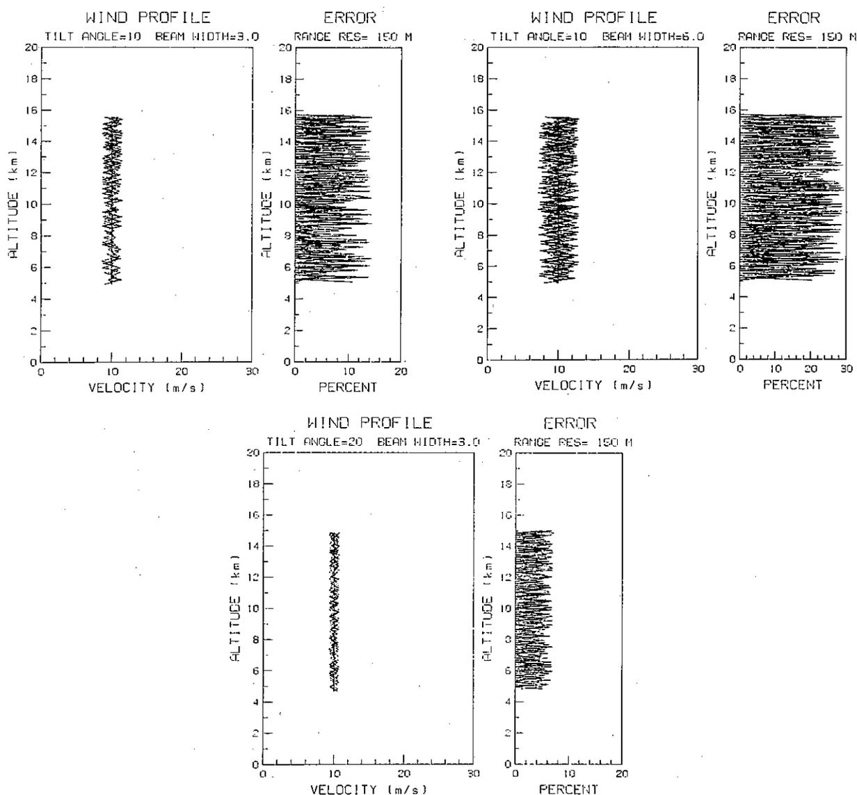
Fig. 2. The model results for a uniform wind profile for radars with a beam width of  $3^\circ$  and tilt angles of  $10^\circ$  and  $20^\circ$  as well as a case for a tilt angle of  $10^\circ$  and a beam width of  $6^\circ$ . The results of 10 simulations are superimposed. The model uses a "rectangular" polar diagram and range-weighting function.
