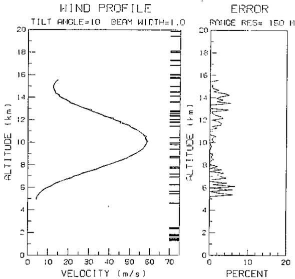
Fig. 6. Model results as in Figure 5, but for an antenna beam width of  $1^\circ$ . Comparing this with Figure 5 illustrates the advantage of using narrow beam widths.
