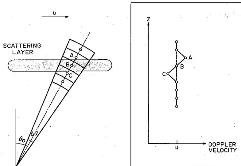
Fig. 1. A geometric representation of the finite range volume effect [after Fukao *et al.*, this issue *a*].
