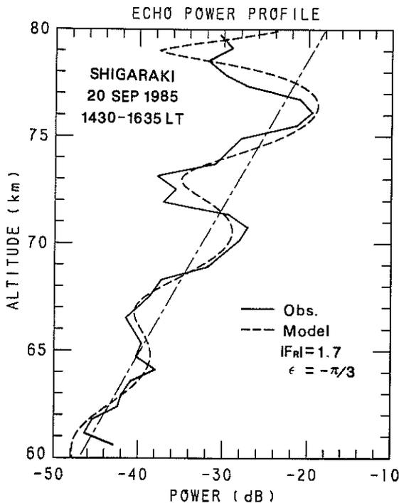
Fig. 3. Comparison of estimated and observed height profiles of normalized mesospheric echo power for 1430–1635 LT on September 20, 1985.
