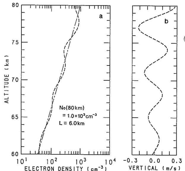
Fig. 4. Height profiles of (a) electron density and (b) vertical wind perturbations estimated from the observed echo power and gravity wind motion summarized in Table 1.
