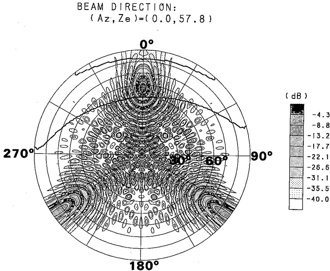
Fig. 5. Contour map of the MU radar relative antenna gain pattern in the beam direction of Figure 4. The thick curves enclose the azimuth-elevation domain of possible perpendicularity between the magnetic field lines and the half-power points of the radar beam for various pointing directions and 50–2000 km range.
