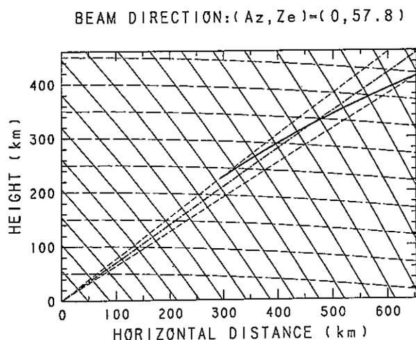
Fig. 4. An antenna beam used for  $F$  region FAI observations that is tilted  $57.8^\circ$  toward due north, and its relation with the locus (thick line) of perpendicularity to  $B$  (thin solid lines).
