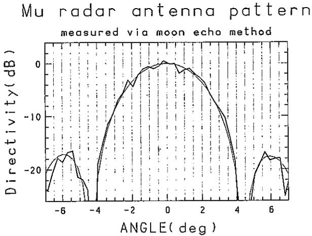
Fig. 1. Relative gain of the MU radar antenna pattern (thick line) measured by moon-reflection echoes and the corresponding theoretical gain (thin line). The antenna beam is tilted by  $8^\circ$  from the zenith and  $40^\circ$  west from the south.
