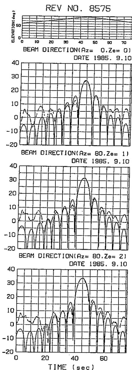
Fig. 3. The MU radar TX antenna patterns (thick broken line) measured by the satellite Ohzora passing around 2° from zenith toward the east, and the corresponding theoretical antenna gain (thin line) relative to the reference antenna. Az is the azimuth angles counted clockwise from the north, and Ze is the zenith angles. The top two patterns show cross-sectional patterns at approximately 2° and 1° from the main lobe peak, respectively.
