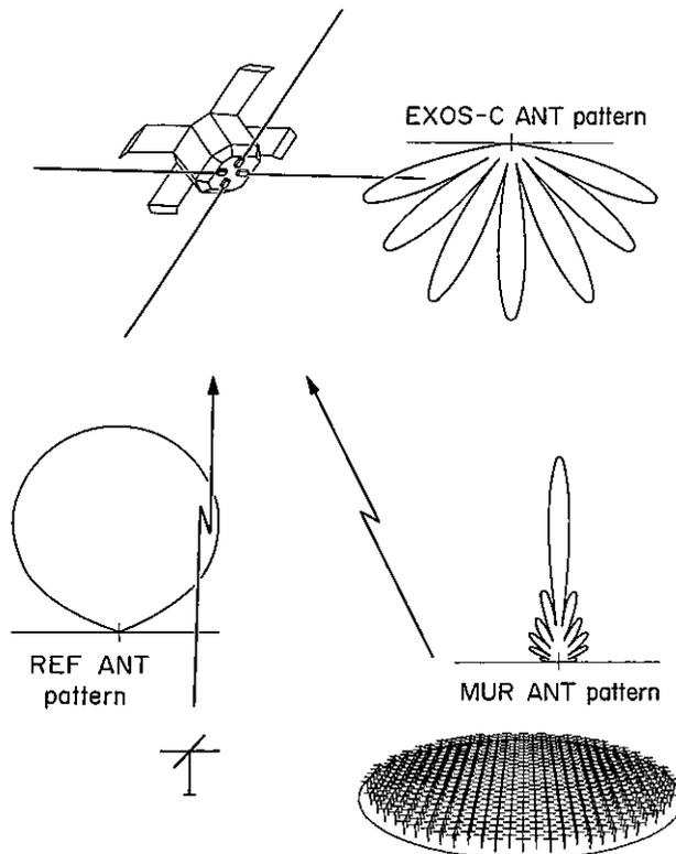
Fig. 2. Principles of the MU radar antenna pattern measurement using the satellite Ohzora. The received signal strength of the MU radar CW signal is calibrated by that of the reference signal strength [Fukao *et al.*, 1985c].
