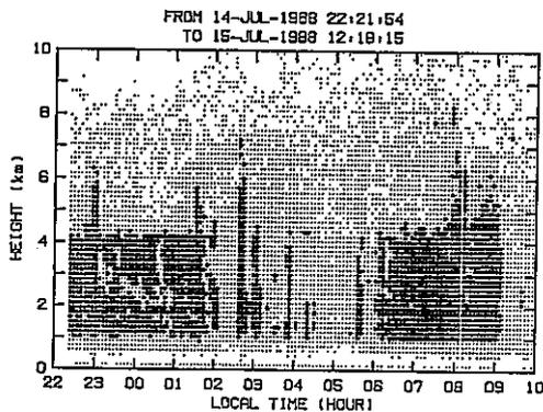
Fig. 8. Detection of echoes by the MU radar. Each dot corresponds to data taken at a time and height interval of 1 min and 150 m, respectively. Large dots denote data points when both the precipitation and turbulence components are identified, and small dots denote that only the turbulence component was detected. Data below about 1.5 km is not reliable because of the reduced receiver sensitivity due to transmit-receive switching.
