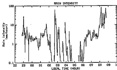
Fig. 7. Temporal variation of the rain intensity measured on the ground at the MU radar site by a drop-counter type rain gauge from 2200 LT, July 14 to 0900 LT, July 15, 1988.
