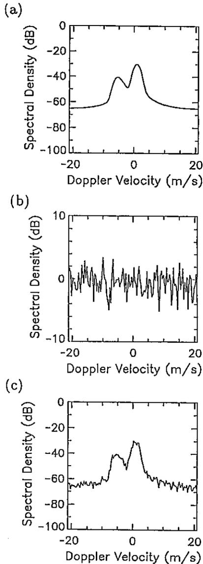
Fig. 1. An example of the model spectra used in the numerical simulation. (a) The theoretical spectra without statistical fluctuations (b) is multiplied by a uniform spectrum with random Gaussian fluctuations (c), resulting in the final model spectrum.
