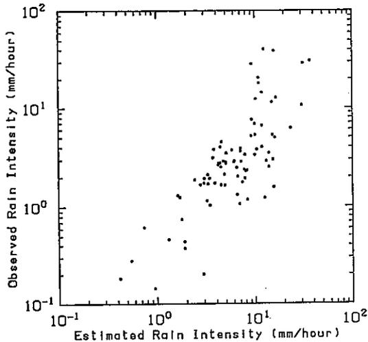
Fig. 10. Correlation diagram of the estimated rain intensity at an altitude range of 1.5–3.6 km by the MU radar and the rain intensity measured at the radar site by the rain gauge for the entire observation period. Each dot denotes an average over 10 min.
