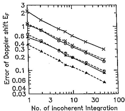
Fig. 6. Error of mean Doppler shift estimated by the standard fitting procedure used for the MU radar data analysis (solid lines) and by the present procedure. Lines with triangle, circle, and cross marks represent the case of  $\sigma = \Delta f$ ,  $3\Delta f$ , and  $10\Delta f$ , respectively.
